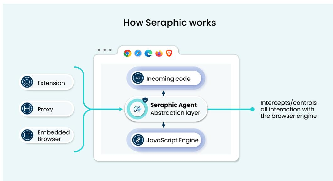
**Figure 7** – The Seraphic Agent can be injected by extension, proxy, or embedded in a dedicated browser. It creates an abstraction layer that can monitor, intercept, and control the interactions between incoming code and the JavaScript Engine.
